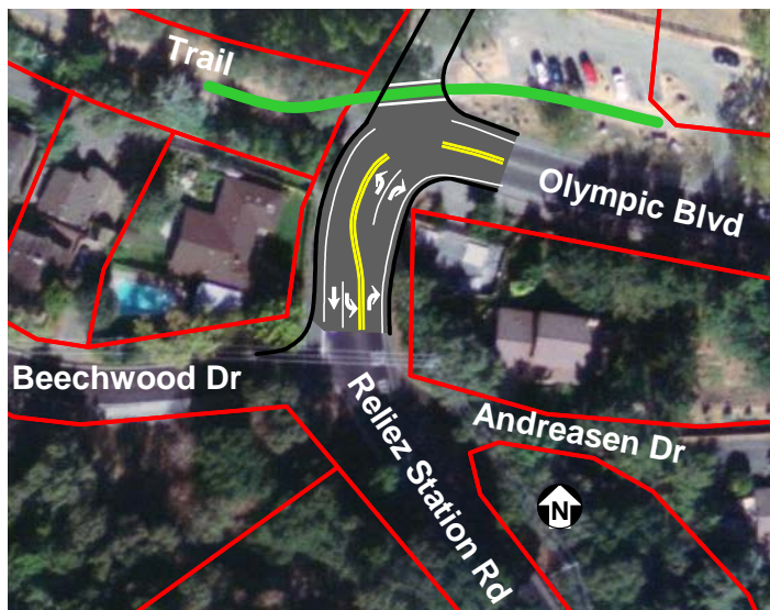
Figure 5: Side Street Stop Control
